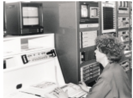
Louise Moss, operator at the York DELC, uses a character generator to broadcast the weekly schedule.
